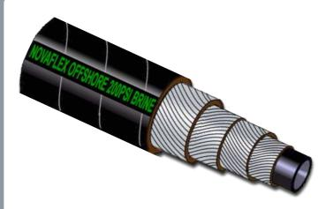
Novaflex Offshore 200psi Brine Hose is used as a bulk transfer hose in the offshore oil and gas industry. Used to transfer from shore to ship and ship to rig the saline liquid usually used in completion operations and when penetrating a pay zone. Brines are used because they have higher densities than fresh water, but have fewer solid particles that might damage production formations.
